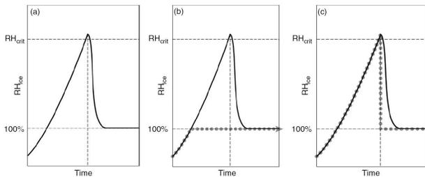
Figure 2. (a) RH evolution in a hypothetical parcel (grid cell) subject to adiabatic cooling at  $T < 235$  K. (b) ECMWF IFS approximation. (c) Ice supersaturation parameterisation by Tompkins *et al.*. The dotted lines in (b) and (c) indicate approximations to (a). [5]
